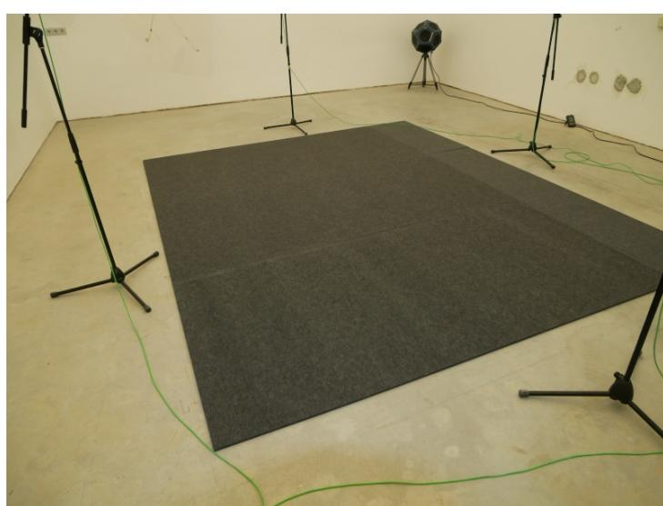
**Picture 6:** Photography of test specimen 2.3 in the reverberation room.
