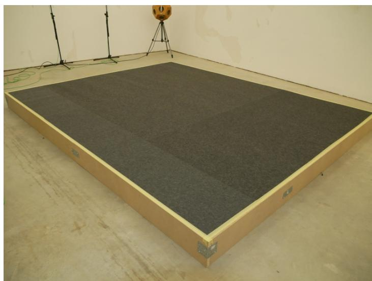
**Picture 2:** Photography of test specimen 2.1 in the reverberation room.
