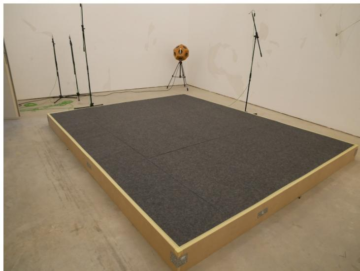
**Picture 1:** Photography of test specimen 1.1 in the reverberation room.
