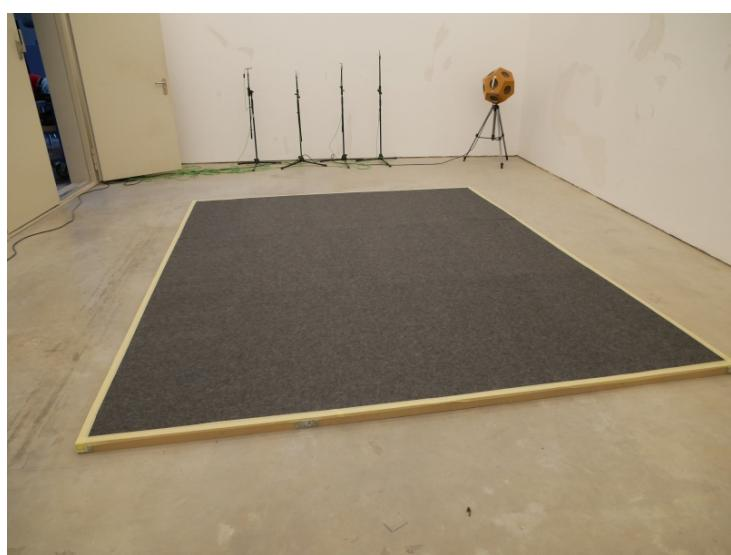
**Picture 3:** Photography of test specimen 1.2 in the reverberation room.
