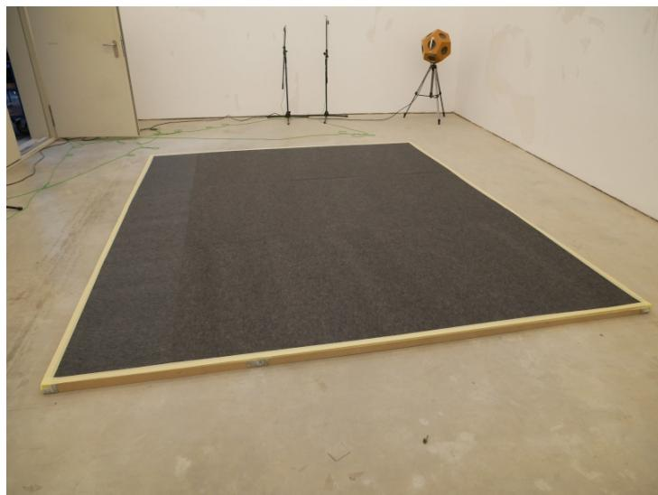
**Picture 4:** Photography of test specimen 2.2 in the reverberation room.
