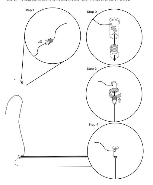
Level the lamp by adjusting the wire. Pull the wire to shorten it or press the tab of the suspension mount to release it. It is recommended that two persons perform this step.
