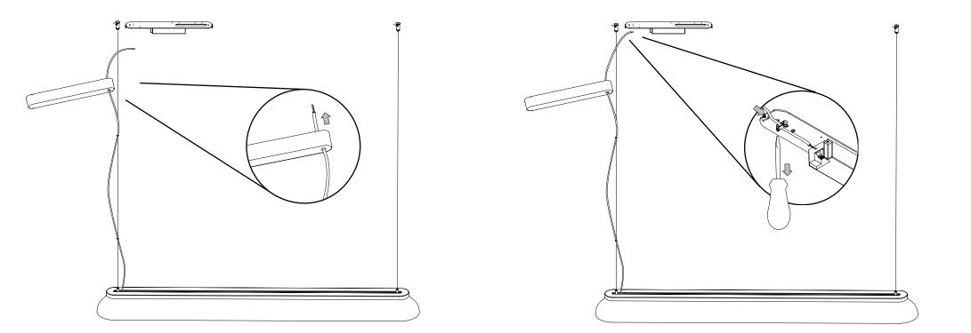
Wiring to mains power: Taking one wire at at a time, insert the correct wires into the corresponding slots on the terminal block, while pressing down on the small button next to them. The live mains wire should be inserted into the slot marked L and the neutral mains wire into the slot marked N. If you are unsure of the polarity of the wires, then we recommend you contact a certified electrician.
