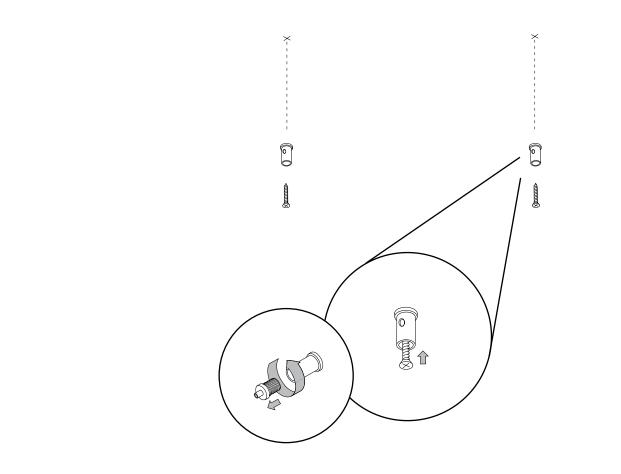
Once the suspension mounts are firmly in place, the lamp is ready to be mounted. Start by pulling the suspension wire through the disassembled suspension mount (step 1). Guide the wire though the fixed suspension mount and through the exit hole on the side (step 2). Screw the disassembled suspension mount together with the part that is fixed to the ceiling (step 3). The suspension wire is now safely in place (step 4). Repeat on the other side.
