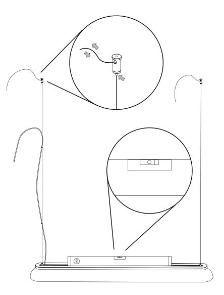
Once the lamp is in place, the excess wire trailing from the exit hole can be cut. Note that once the wire has been cut, the lamp can no longer be lowered.
