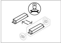
**A** The light source of this luminaire is not replaceable. When the light source reaches its end of life the whole luminaire shall be replaced.
