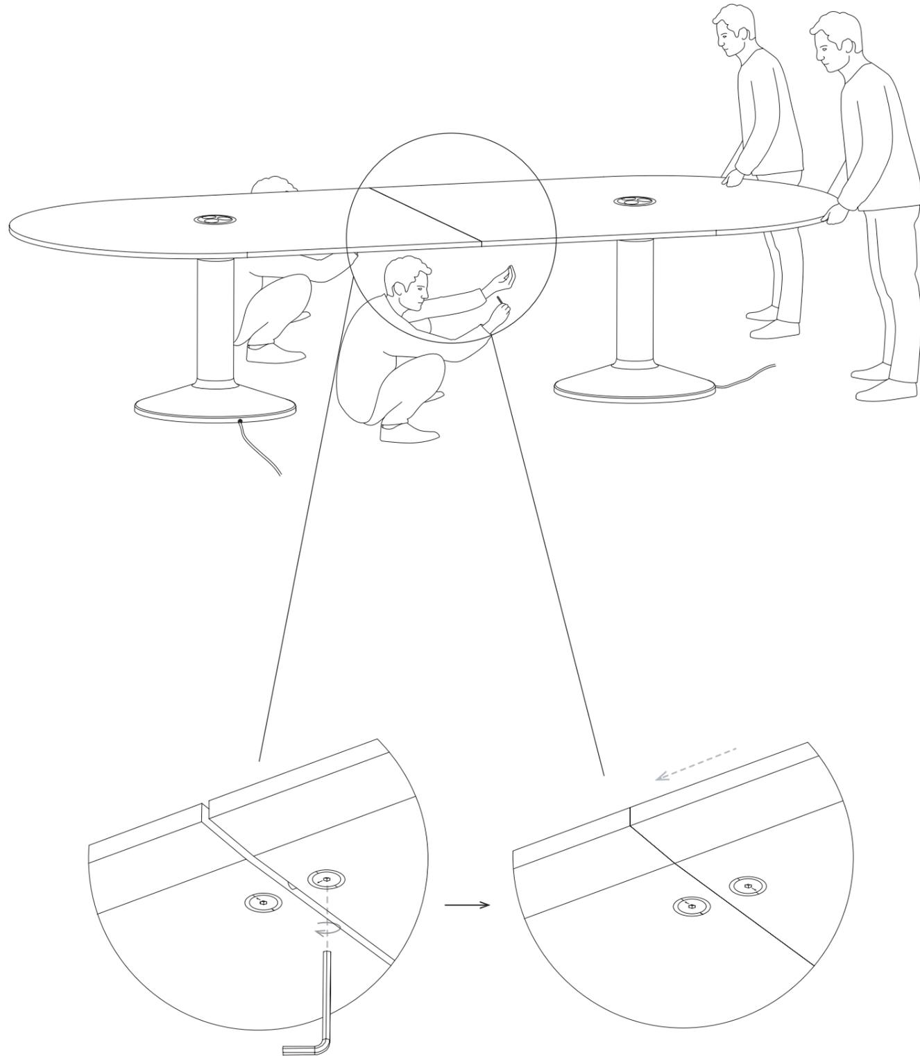
Simultaneously tighten the 2 round fittings on the 2nd half of the tabletop.
