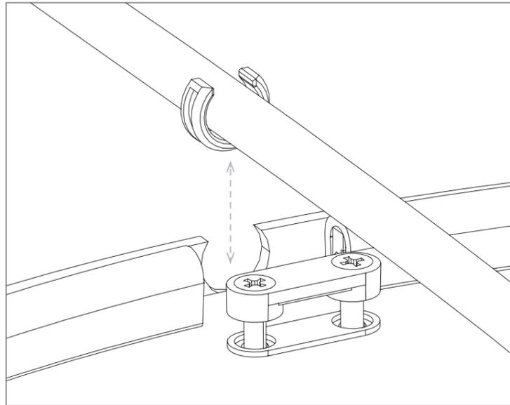
The pre-mounted black rubber cable protection must always be fixed to the outer edge of the base. An extra one is included with the screws.
