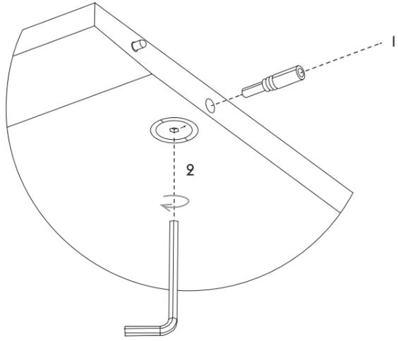
Place one of the metal dowel pins through the tabletop into the round fitting. Use the key provided to tighten the dowel pin. It should retract into the tabletop with each turn. Keep turning until tight and the pin head is flush with the tabletop edge.
