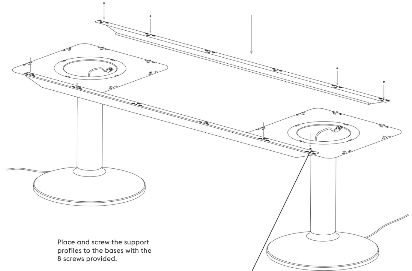
Place and screw the support profiles to the bases with the 8 screws provided.
