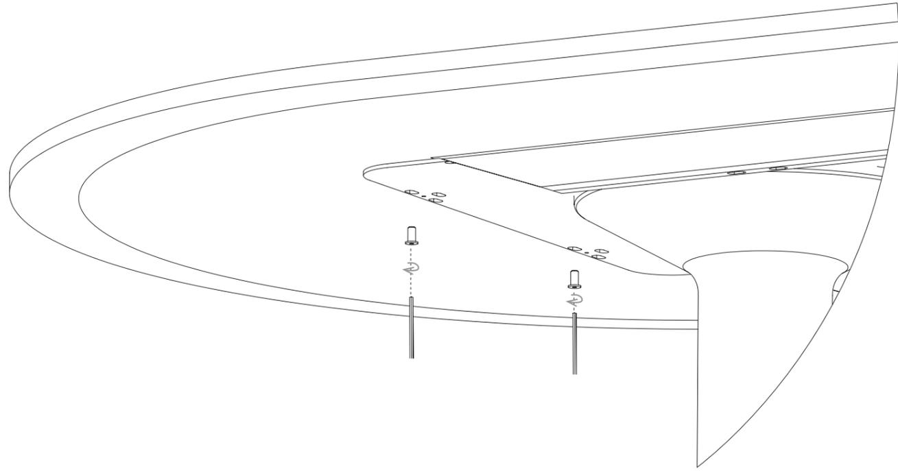
Secure the tabletop by placing a few tabletop screws. Do not over tighten.
