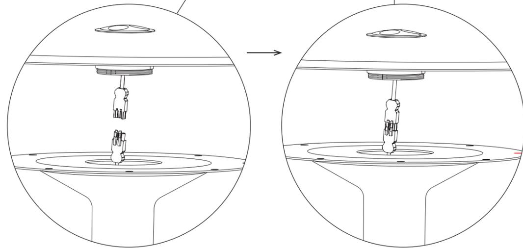
Connect the cable from the base to the power unit mounted in the tabletop.
