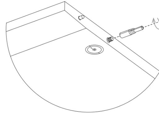
Connect the next dowel pin to the thread. Turn until tight.
