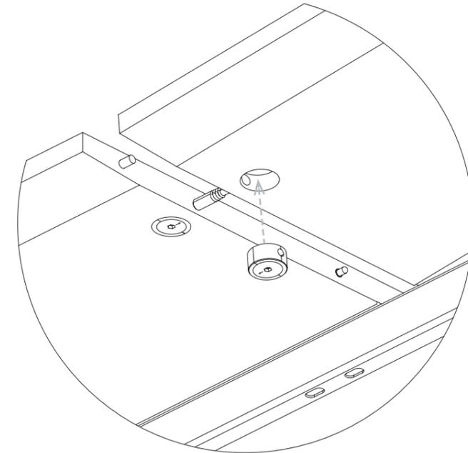
Place the round fittings into the circular cutout under the table so the arrow and larger holes are facing in the same direction and towards the pin on the opposite side.
