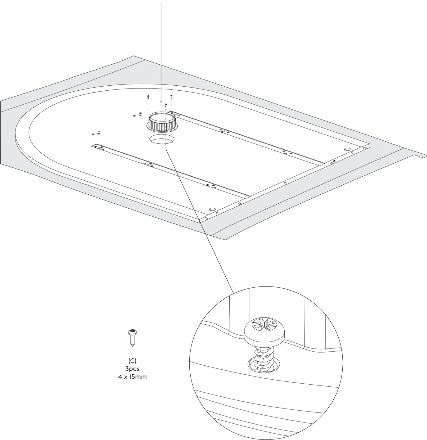
Screw the power units to the locking rings in the tabletop until secure.
