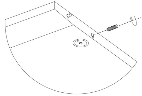
Connect the threaded pin to the dowel in the tabletop. Turn completely until tight.
