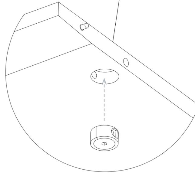
Place the round fitting into the circular cutout under the table so the arrow and larger hole are facing in the same direction and towards the centre of the tabletop.
