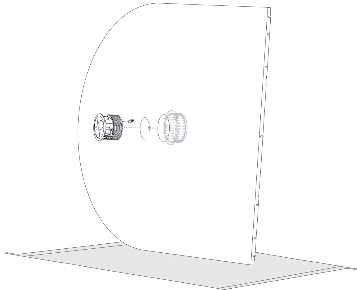
8 As 2 people lift the tabletop above the base, a third person should connect the cable from the base to the power unit mounted in the tabletop.
