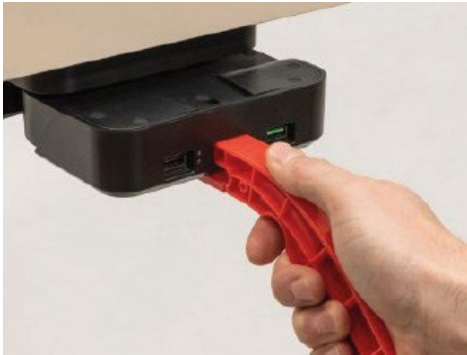
A magnetic key allows you to unlock the battery and extract it in a jiffy to recharge it.
